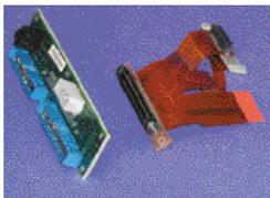
**Adapter module and flex etch**
