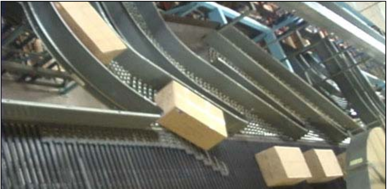
SDI’s deliverables to Liz Claiborne included carton conveyor systems and two high-speed carton sorters.
